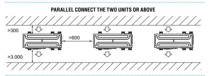
PARALLEL CONNECT THE FRONT WITH REAR SIDES
